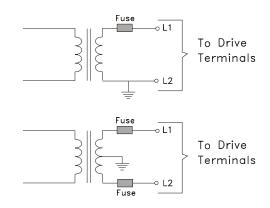
Figure 10: Single Phase Power Supply Connections
